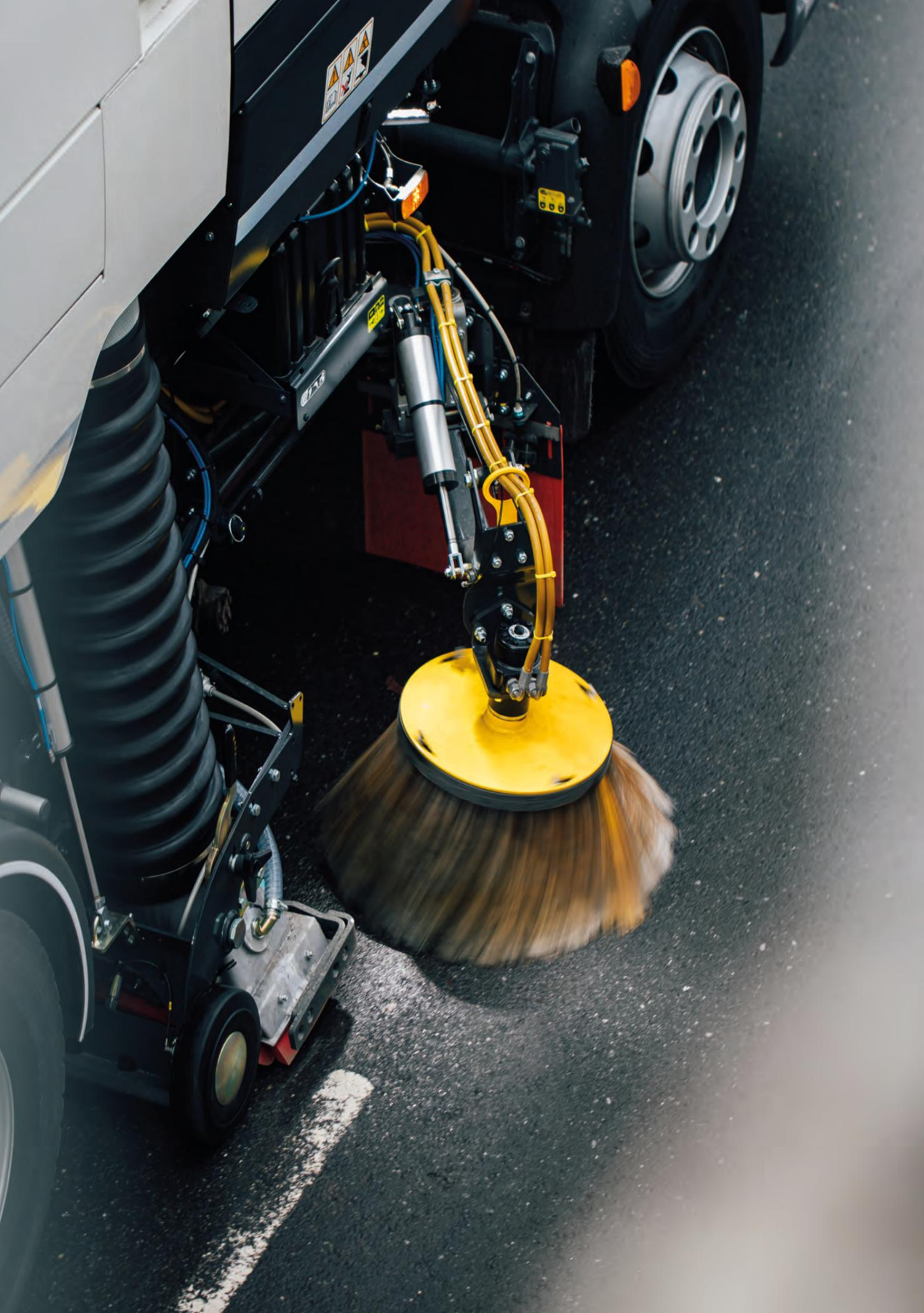
A close-up, high-angle photograph of a street sweeper's brush assembly. The brush is a large, circular, yellow-tipped roller with dense, brown bristles, mounted on a mechanical arm. The arm is connected to a complex system of hydraulic lines and hoses. The machine is positioned on a dark asphalt surface, and a white painted line is visible on the ground. The lighting is dramatic, highlighting the textures of the brush and the metallic components of the machinery.
