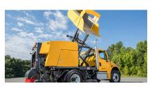
Ultra High Dump providing an additional 0.5m (18inch) tip height ideally suited to transferring debris into a tipper truck.
